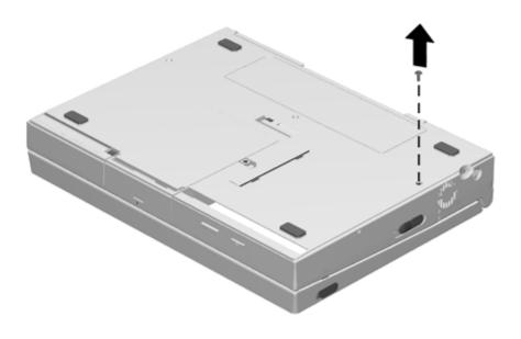
Figure 5-12. Removing the MultiBay Security Screw
